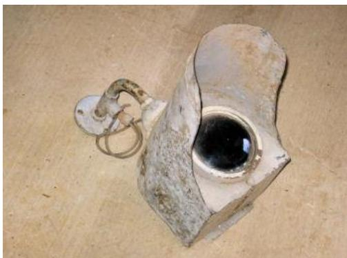
At the exit to each block is a single aspect green signal which is also linked in series with the previously mentioned signals. The purpose of this signal is to indicate that once the tram leaves the block the signals are also cleared from the indicators. If however the green light remains on after the passage of the wheel under the switch, it conveys that a following car has also entered the block.
