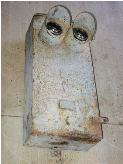
The motorman of a tram approaching a single track section will know that his car will have sole occupancy of this section if no lights are shown on the indicator. On proceeding, the trolley wheel passes under the switch and a green light is registered on the indicator at the point of entry. Simultaneously a red warning light is cut in at the opposite end of the block.
